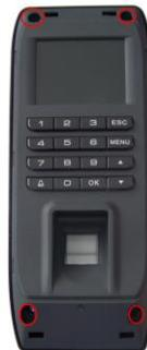
Noted: Fasten the orientation template on the wall first, and put the sealing ring on, then install the device.
